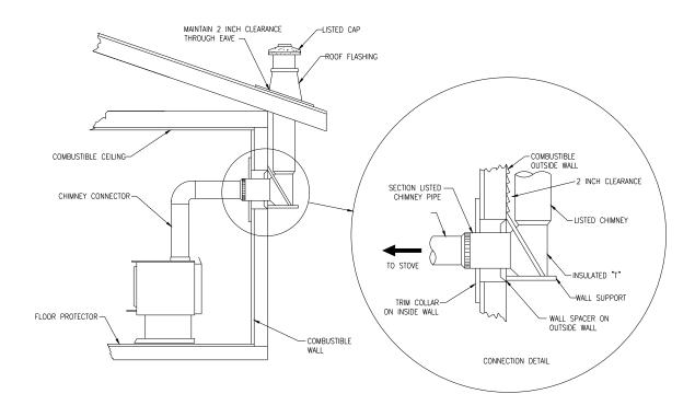
FIGURE 2.2.1 (A) Typical installation through the wall
